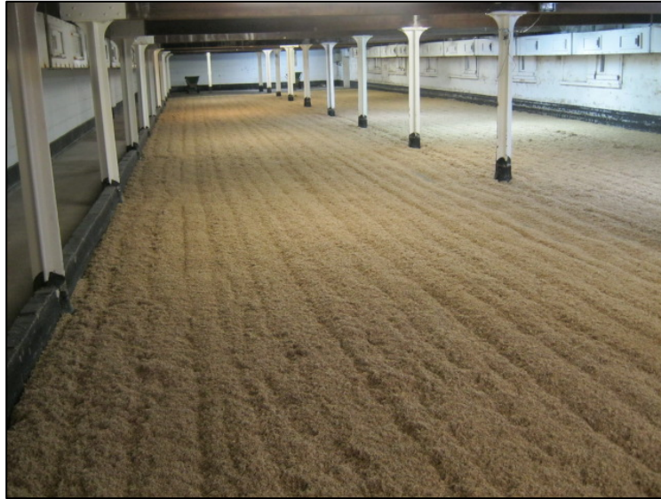
Figure 2.2 Germination floor at a traditional (19th century) floor maltings at Crisp Malt, Great Ryburgh, northwest Norfolk (photograph: August 2019)
